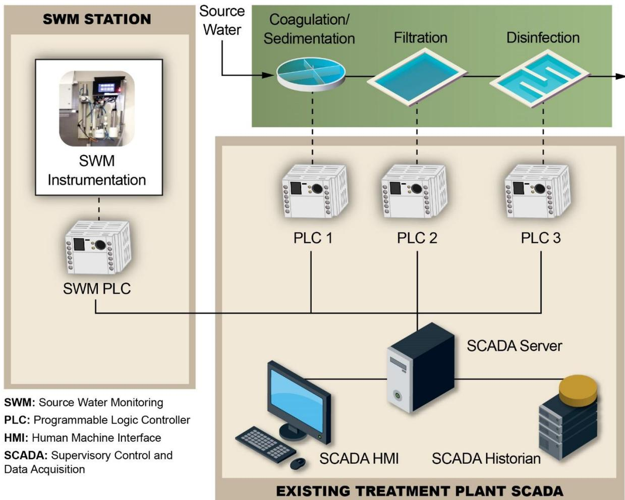
**Figure 6-7. SWM Information Management as an Extension of an Existing SCADA Architecture**
