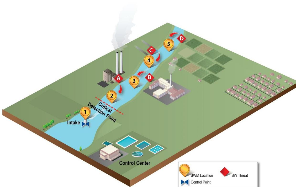
**Figure 3-3. Multiple Upstream SWM Locations to Monitor Multiple SW Threats**
