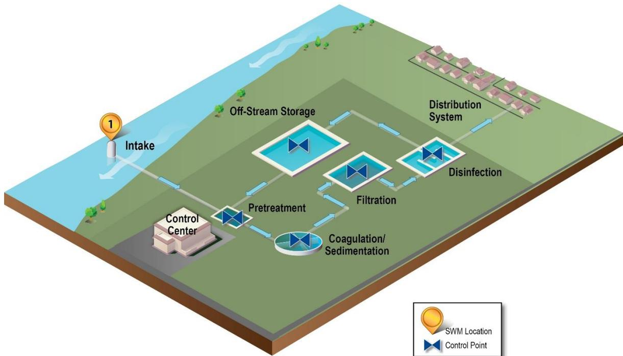
**Figure 3-1. SWM Location Selected to Support Treatment Process Optimization**
