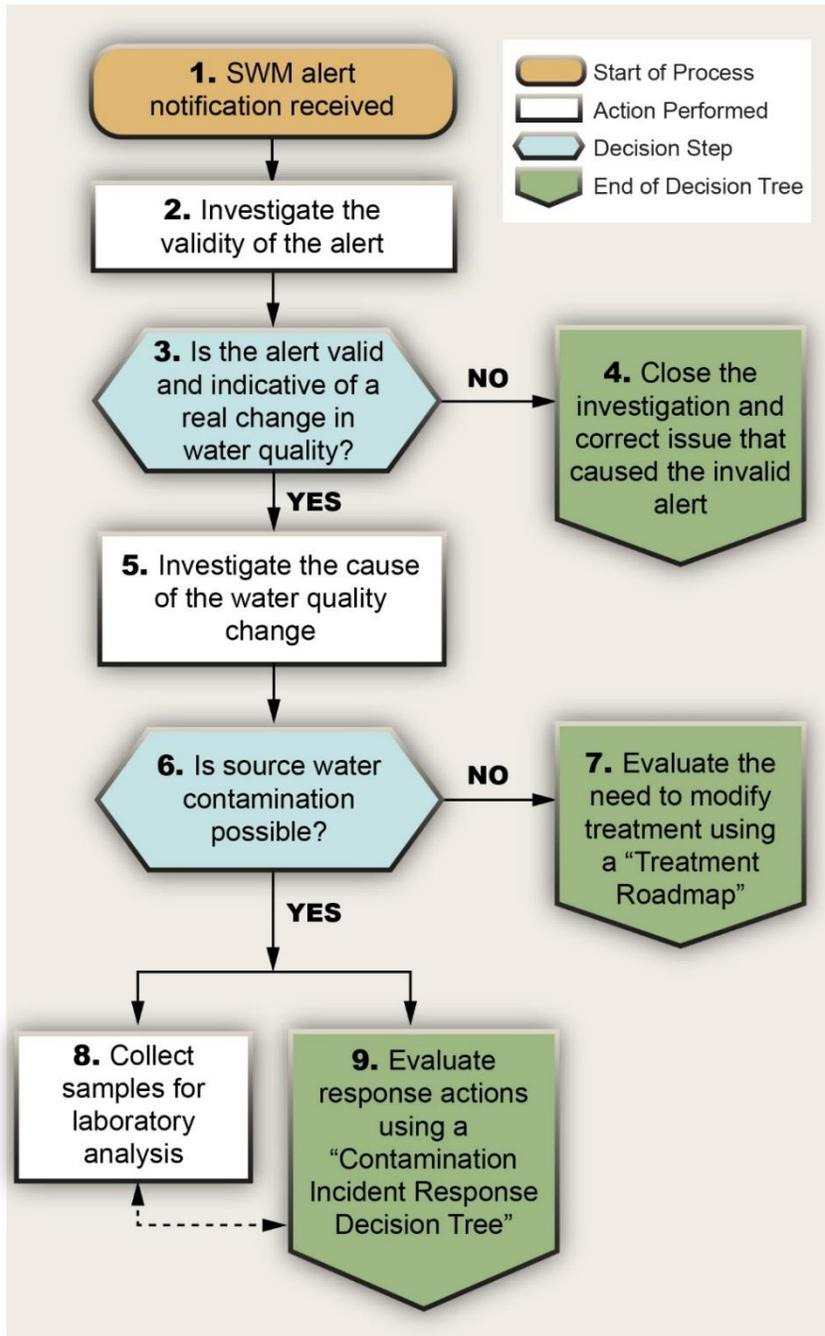
Figure 7-1. Example of an SWM Alert Investigation Process Flow Diagram
