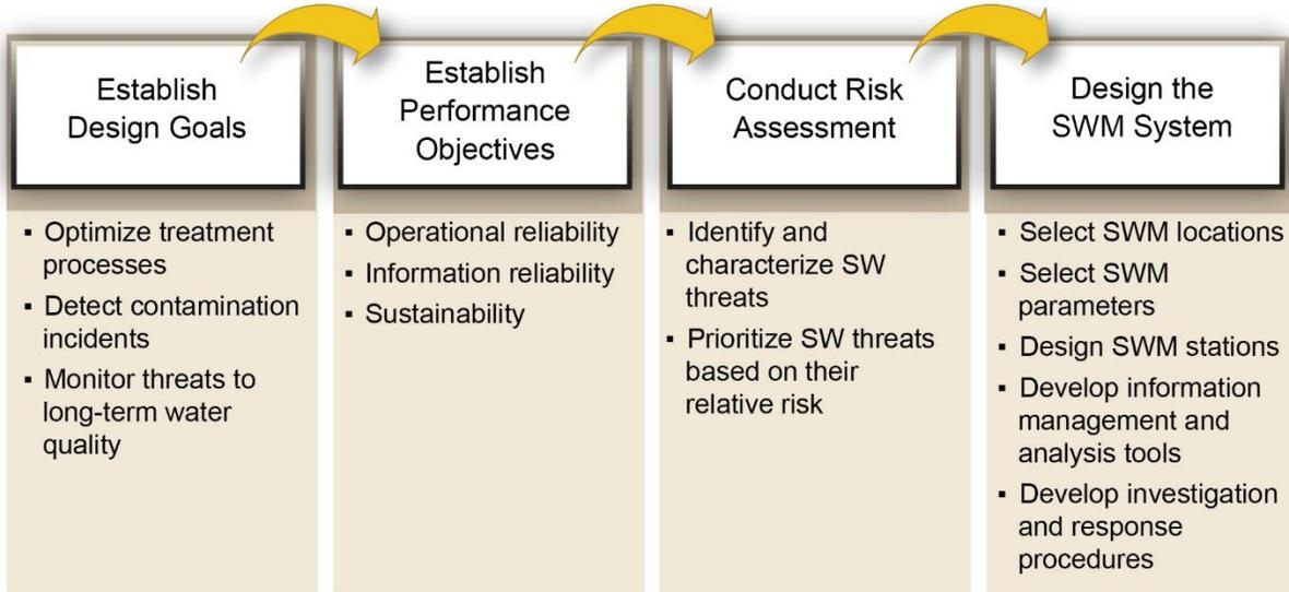
**Figure 2-1. Source Water Monitoring Implementation Framework**
