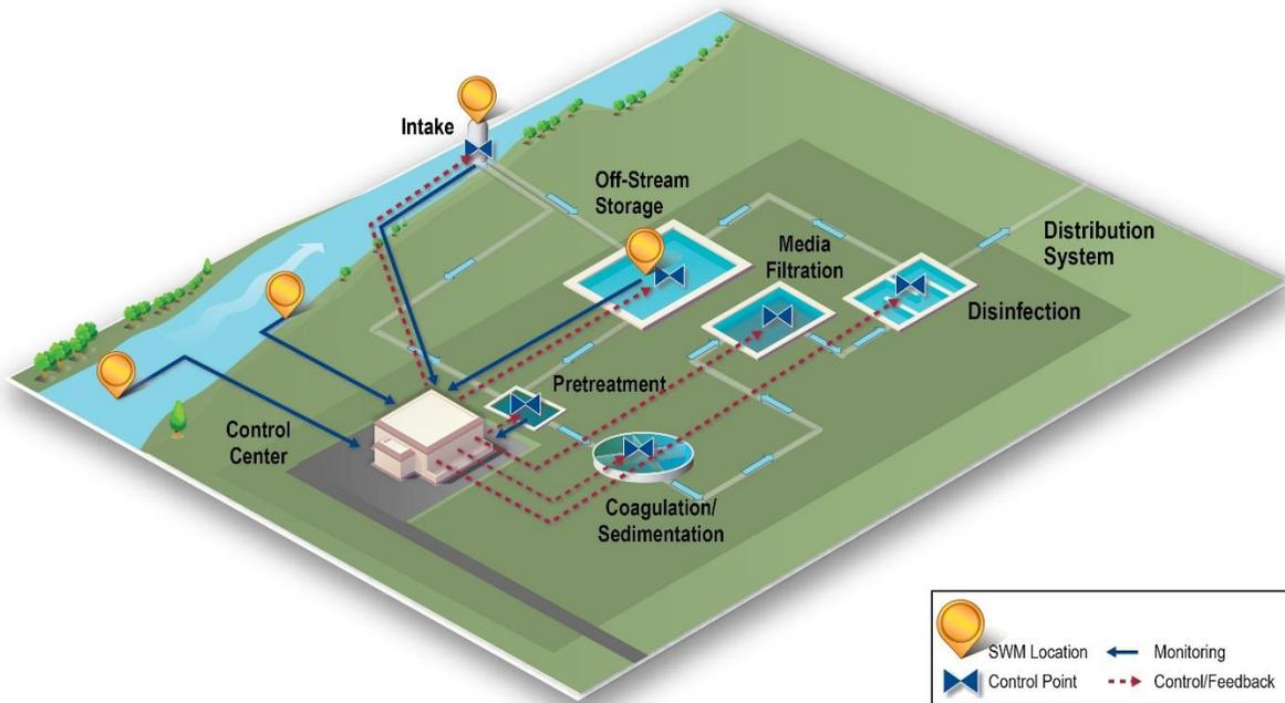
Figure 1-2. Example Schematic of Source Water Monitoring
