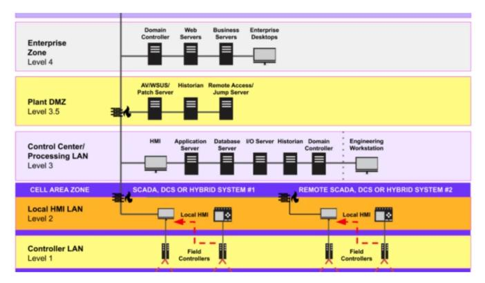
This diagram shows the standard architecture of an industrial network configured according to the Purdue Model. Industrial devices are located at levels 0 through 3.4
