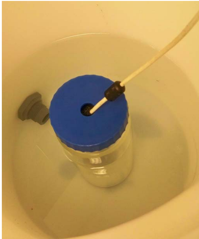
Figure 2-12 Encased 3 × 3 inch NaI detector submersed in 20 liter K-40 solution.
