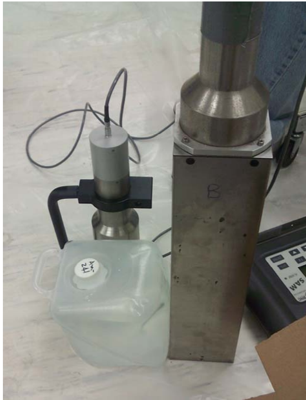
Figure 2-9 Encased 3 × 3 and 4 × 16 inch NaI detectors against 4 liter Am-241 sample.
